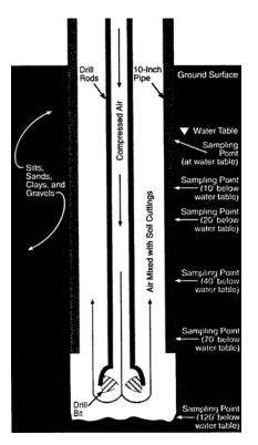
DIAGRAM OF DRILL-BIT & BOREHOLE:
